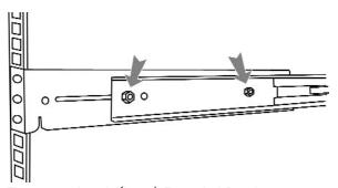
Figure 48 Attach (Long) Extended Brackets
